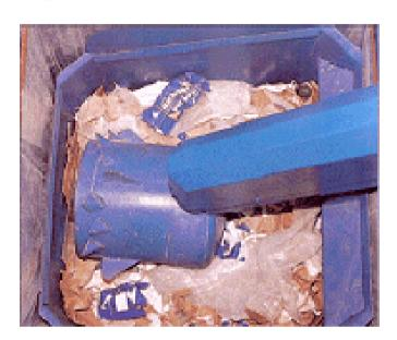
A Rotary Waste Compactor takes up little more space than a standard wooden pallet, yet amazingly can compact the entire contents of a waste skip into one polythene wastebag.
